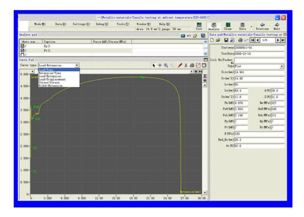
Multiple curves function in real time display including Load-Extension, Load-Displacement, Stress-Strain, Load-Time, Extension-Time, and Width-Extension.
