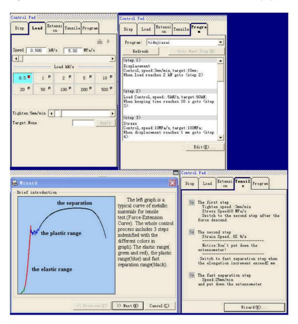
Through the Tensile Program Editor, user can setup test steps according to the requirements of standards.
