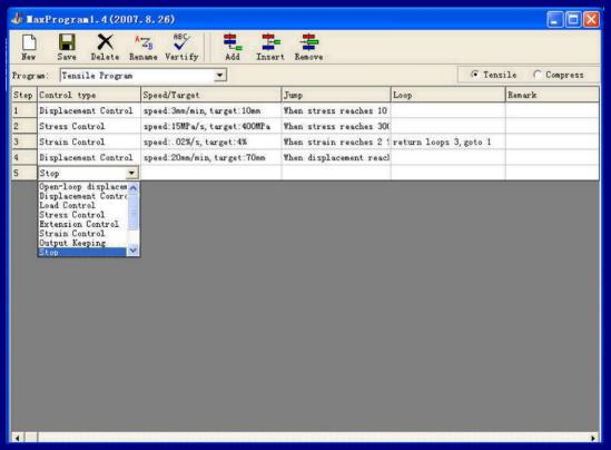
MaxProgram Editor possesses of multiple full digital control modes, i.e Displacement control, Stress (Load) control, Strain (Deformation) control, Low cycle control. User can edit the most complex and logical procedure by MaxProgram Editor. The combination of above functions can meet all kinds of routine test purpose.
