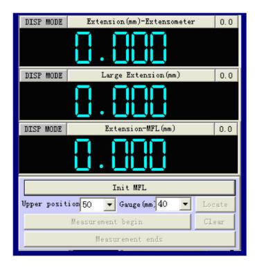
Except the clip-on Extensometer, TE software supports Long Travel Extensometer, Full Automatic Extensometer, video Extensometer, laser Extensometer, and it can be added eight Extensometers at most.
