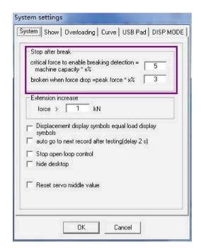
Overload protection function & Break detection functions can be set through software
