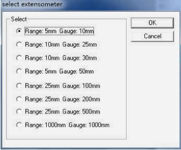
Except the clip-on Extensometer, TE software supports Long Travel Extensometer, Full Automatic Extensometer, video Extensometer, laser Extensometer, and it can be added eight pieces of Extensometers & eight pieces of load cells at most.
