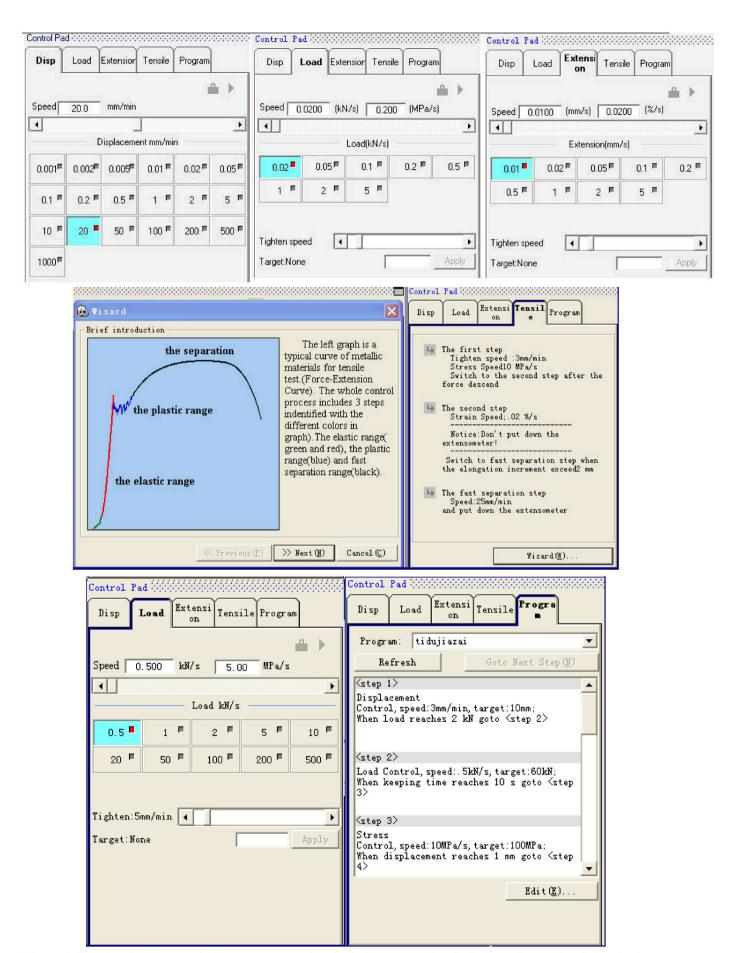
Through the Tensile Program Editor, user can setup test steps according to the requirements of standards.
