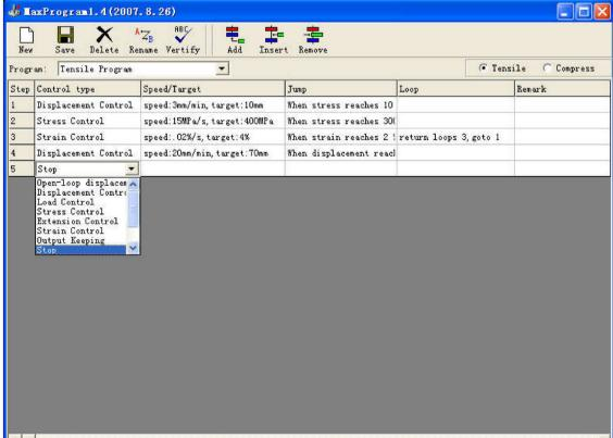
MaxProgram Editor possesses of multiple full digital control modes, i.e Displacement control, Stress (Load) control, Strain (Deformation) control, Low cycle control. User can edit the most complex and logical procedure by MaxProgram Editor. The combination of above functions can meet all kinds of routine test purpose.
