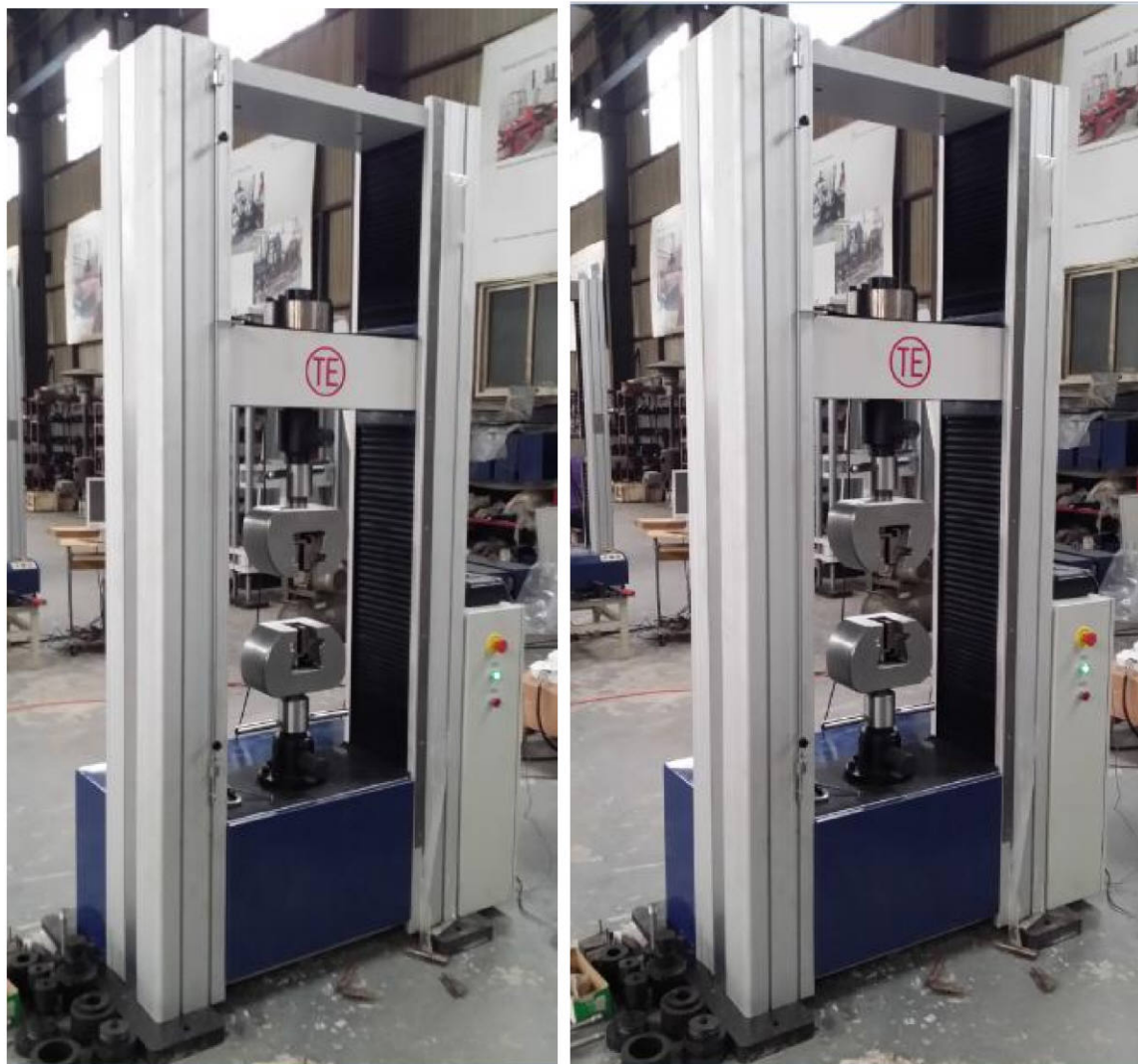
Load Frame of this WDW-300S Superior machine
