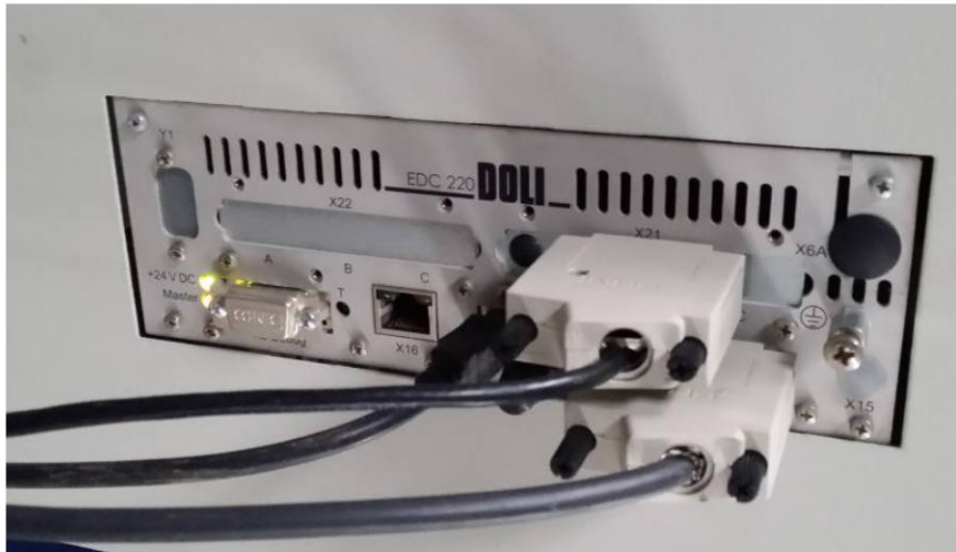
Advanced EDC 220 Controller from Doli, Germany with 1000Hz sampling rate
