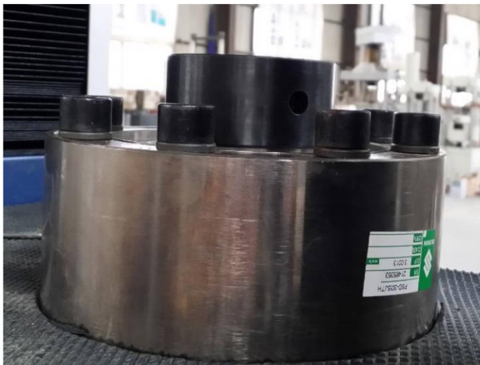
Advanced Load Cell from Celtron, USA
