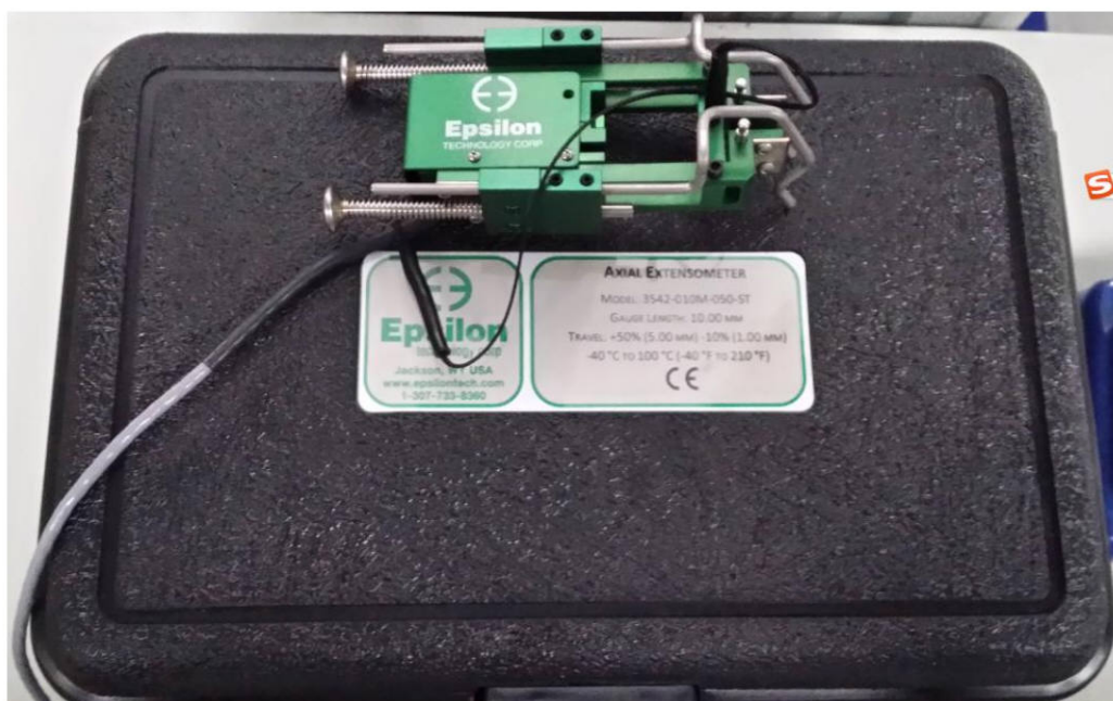
Epsilon Extensometer Model 3542-010mm-050-ST used for strain control function as per ISO 6892 Method A
