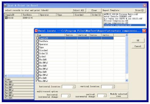
TE software contains all kinds of Report Templates. Customer can design various testing reports according to the requirements. Test result and curve can be converted to ASCII or spread sheet or Excel or the auto-creating report template.
