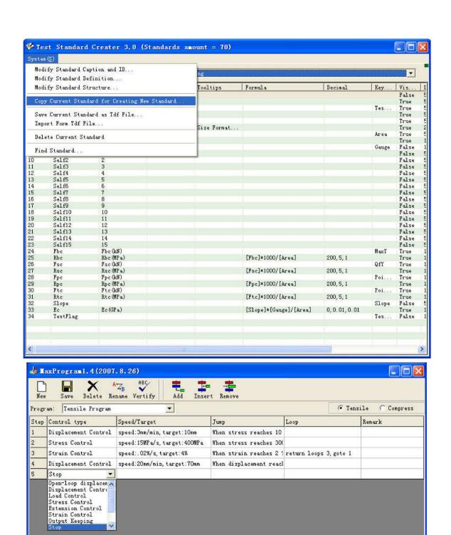
MaxProgram Editor possesses of multiple full digital control modes, i.e Displacement control, Stress (Load) control, Strain (Deformation) control, Low cycle control. User can edit the most complex and logical procedure by MaxProgram Editor. The combination of above functions can meet all kinds of routine test purpose.
