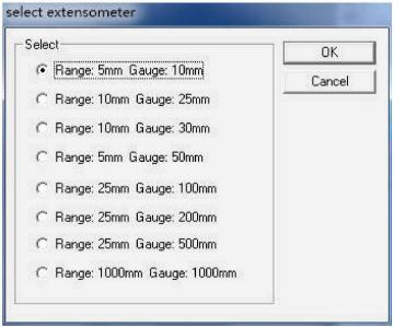
Except the clip-on Extensometer, software supports Long Travel Extensometer, Full Automatic Extensometer, video Extensometer, laser Extensometer, and it can be added eight pieces of Extensometers & eight pieces of load cells at most.
