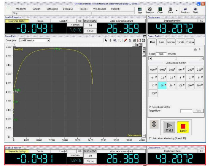
5-digit display for load, peak value and displacement values at least, 4-digit display for extension value at least;
