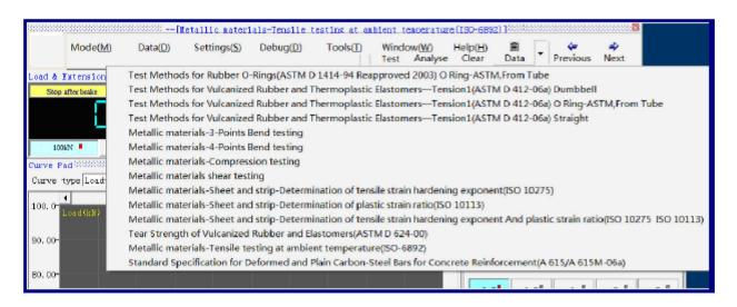
Software supports all kinds of popular testing standards i.e. ISO, ASTM, BS EN, DIN, JIS, GB etc. Users can modify and add own testing standards and methods.
