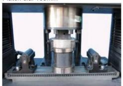
3 points Flexural test fixture:
