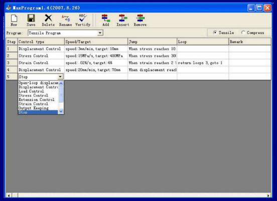
MaxProgram Editor possesses of multiple full digital control modes, i.e Displacement control, Stress (Load) control, Strain (Deformation) control, Low cycle control. User can edit the most complex and logical procedure
