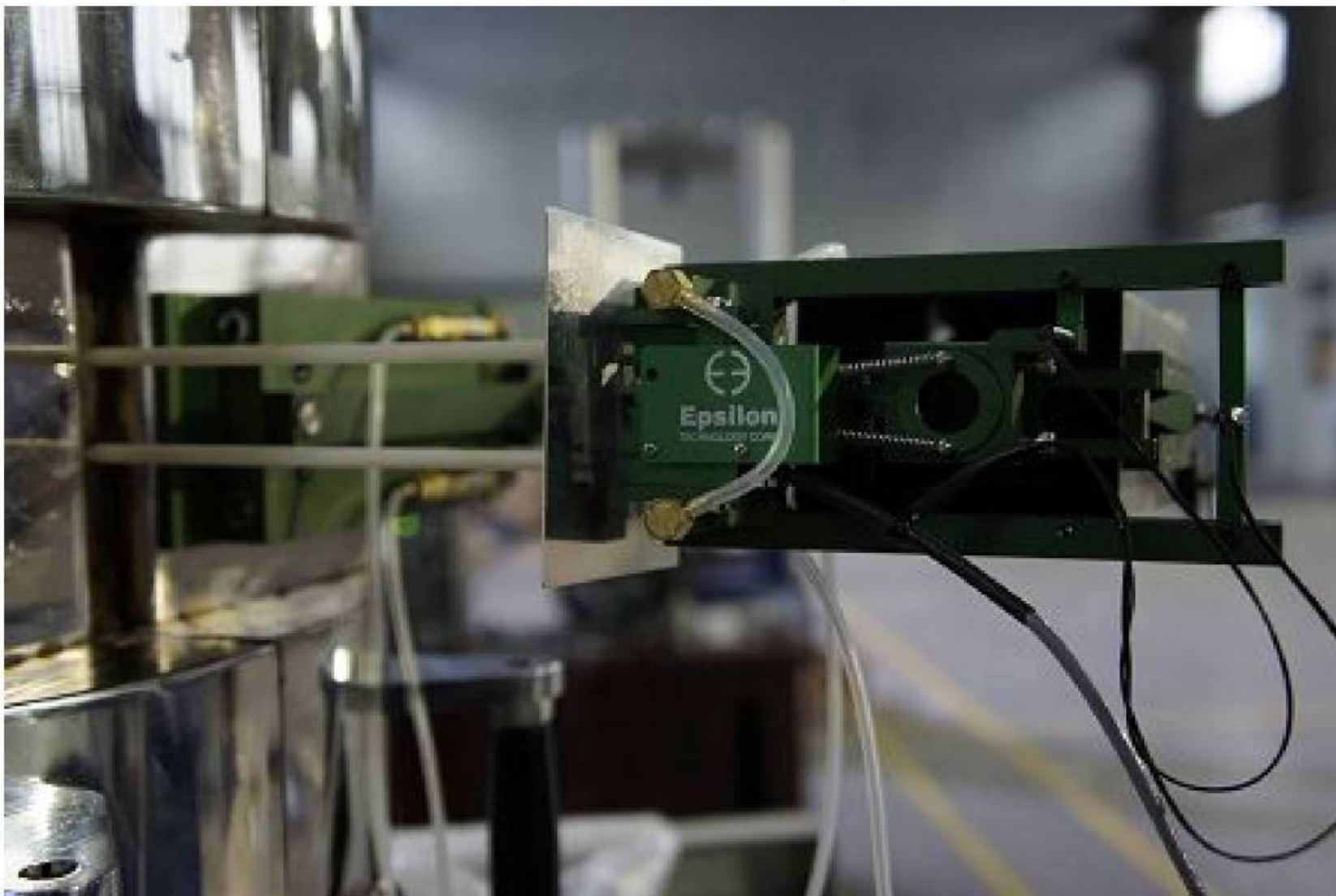
High temperature extensometer Model 3548HI-025M-050-ST from Ms. Epsilon, USA
