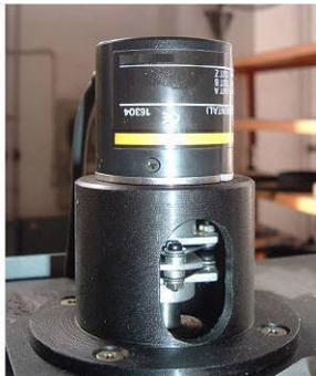
6. Electronic Extensometer for test in room temperature
