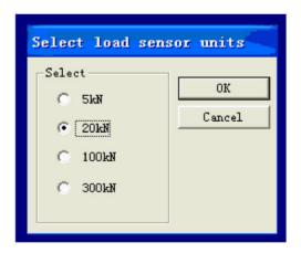
software supports four load cells.
