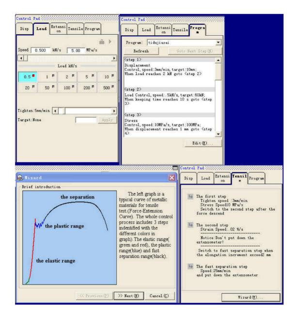
Through the Tensile Program Editor, user can setup test steps according to the requirements of standards.
