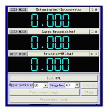
Except the clip-on Extensometer, software supports Long Travel Extensometer, Full Automatic Extensometer, video Extensometer, laser Extensometer, and it can be added eight Extensometers at most.
